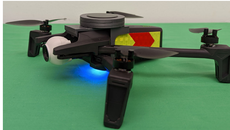
3D Printed Harness 14 g Total Flight Weight 360 g
